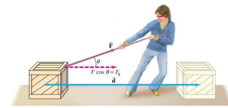
**FIGURE 6–1** A person pulling a crate along the floor. The work done by the force  $\vec{\mathbf{F}}$  is  $W = Fd \cos \theta$ , where  $\vec{\mathbf{d}}$  is the displacement.
