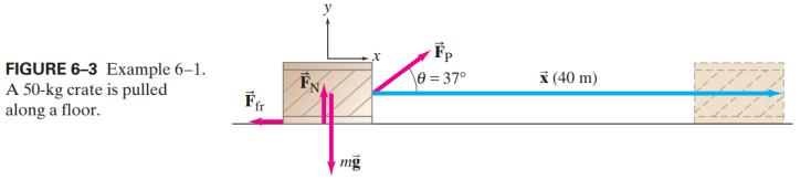
**EXAMPLE 6–1** Work done on a crate. A person pulls a 50-kg crate 40 m along a horizontal floor by a constant force  $F_{\rm P} = 100$  N, which acts at a 37° angle as shown in Fig. 6–3. The floor is rough and exerts a friction force  $\vec{\mathbf{F}}_{\rm fr} = 50$  N. Determine (*a*) the work done by each force acting on the crate, and (*b*) the net work done on the crate.
