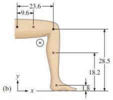
FIGURE 7–26 Example 7–13: finding the CM of a leg in two different positions using percentages from Table 7–1. (⊗ represents the calculated CM.)
