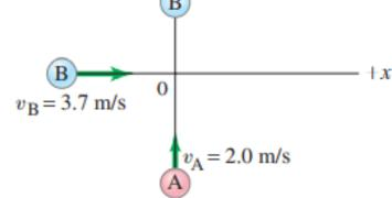
46. Write momentum conservation in the x and y directions and KE conservation. Note that both masses are the same. We allow  $\vec{\mathbf{v}}_{\mathbf{A}}$  to have both x and y components.
