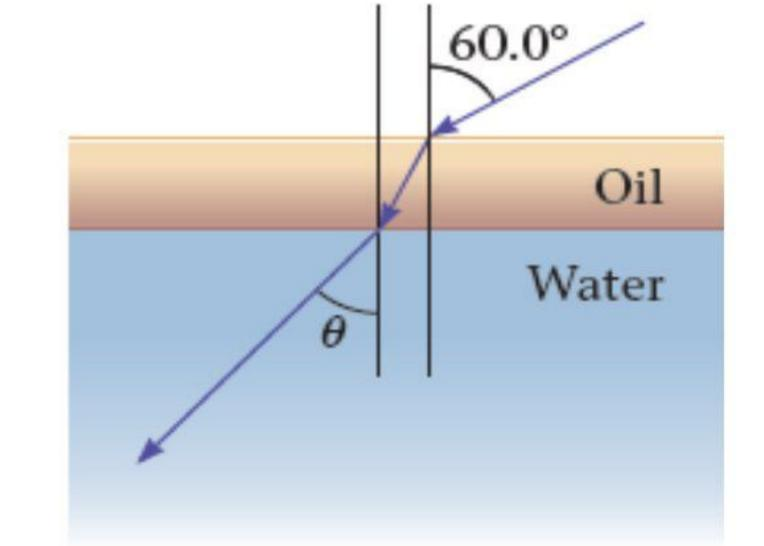
Answer: (a) Because the air/oil and oil/water interfaces are parallel, the angle of refraction at the air/oil interface will equal the angle of incidence at the oil/water interface. Write Snell's law at the air/oil interface and at the oil/water interface, and then combine the two equations and solve for the angle of refraction in water:
