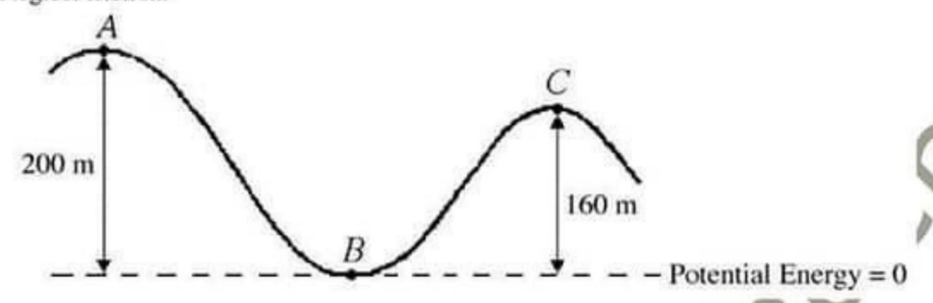
(a) What is the total mechanical energy of the roller coaster at point B?
