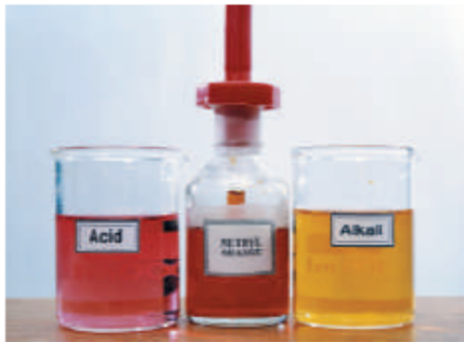
Methyl orange indicator in basic solution (right) and in acidic
