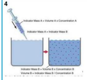
Volume B =  $\frac{\text{Volume A} \times \text{Concentration A}}{\text{Concentration B}}$
